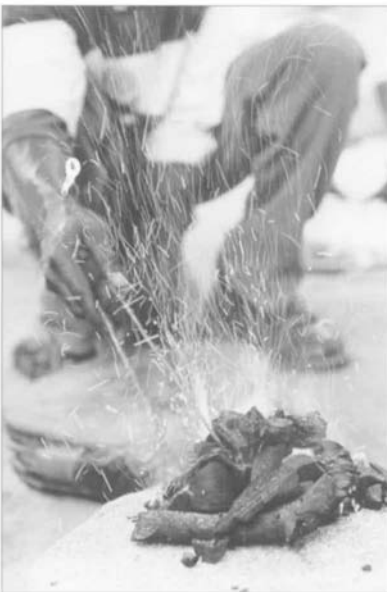
The miners dig pits and shafts between 2m and 15m in depth. The gold-bearing mud is washed, and mercury used to extract the gold and shape it into 'bush gold', which is then smelted over a makeshift furnace.
