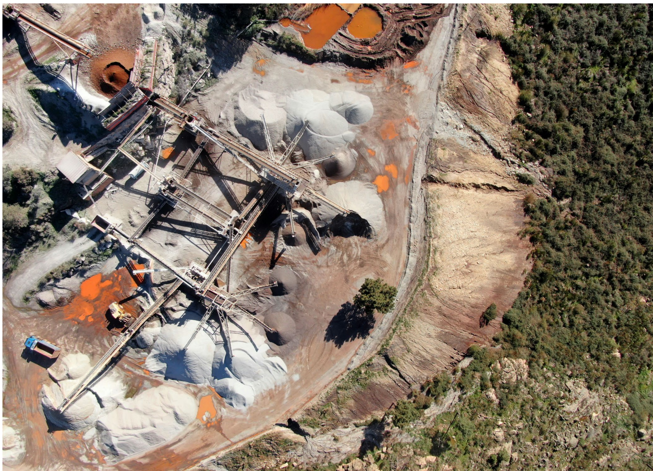
Aerial image of crushing and washing of gravel iron ore at a quarry in Felgar, Municipality of Torre de Moncorvo, Portugal
