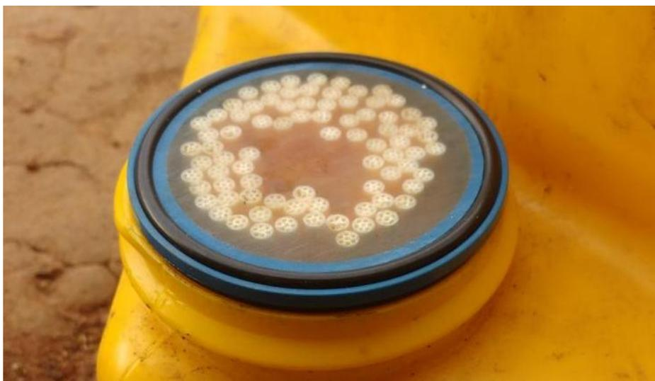
The top of the membrane filter and one of the O-rings which can easily be lost if the cap on the filter side is unscrewed. Photo Credit: Angus McBride / Oxfam
