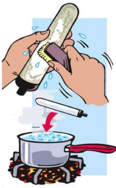
Figure 7: Cleaning of ceramic candles source: IFRC
