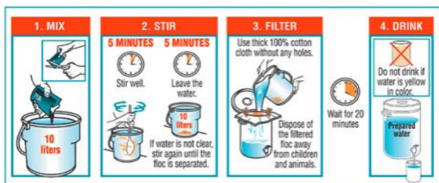
Figure 4: Instructions for use of PUR
