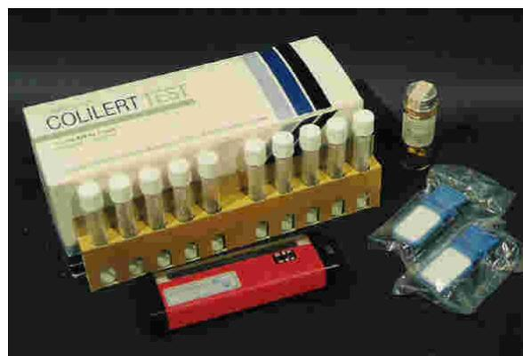
(l-r) Colilert test tubes and fluorescent light; H<sub>2</sub>S strips; Dipslides
