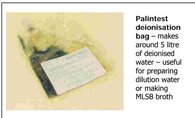
**Palintest deionisation bag** – makes around 5 litre of deionised water – useful for preparing dilution water or making MLSB broth
