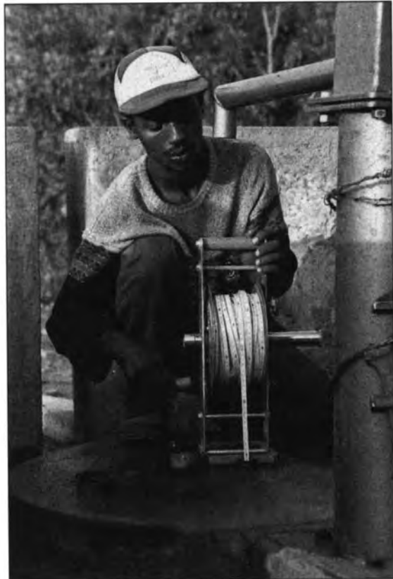
Wolayta, Ethiopia. Measuring the water depth in a well can be made easy.
