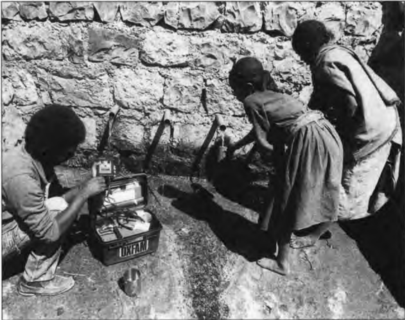
Wollo, Ethiopia. Bacteriological water quality can be tested in remote rural areas using a portable test kit
